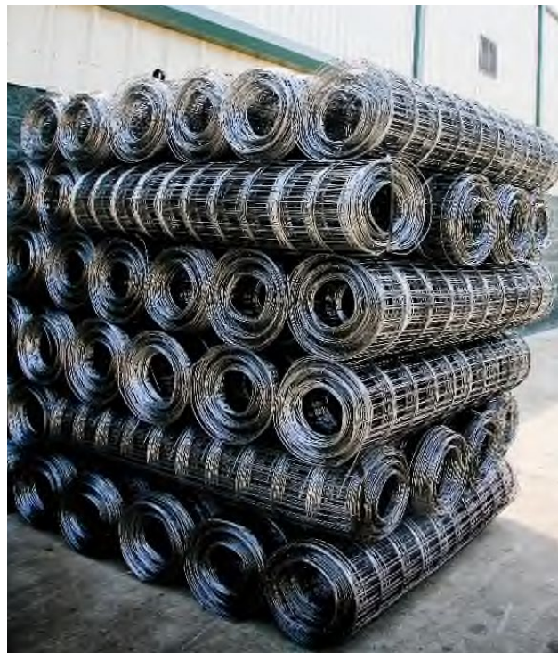
A stack of wire mesh rolls with each fastened from unrolling with steel strapping.
