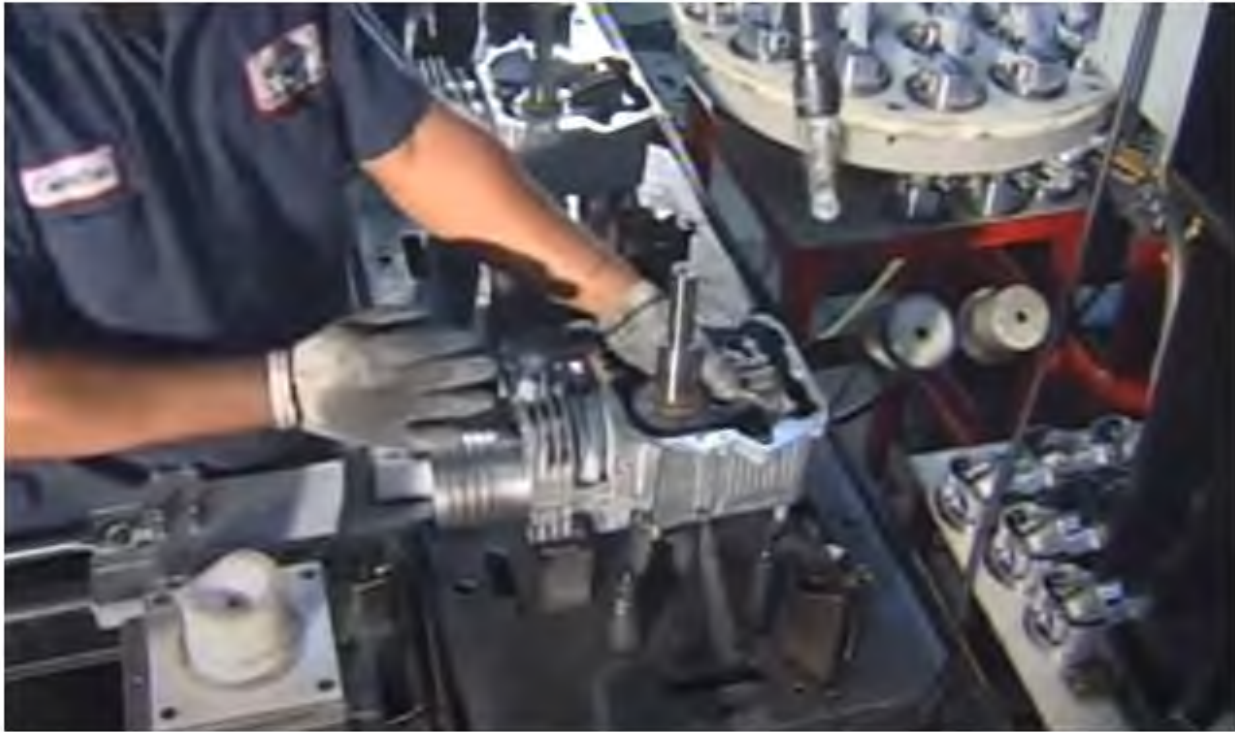
Figure I-6 SVSEs: Piston installed into the cylinder
