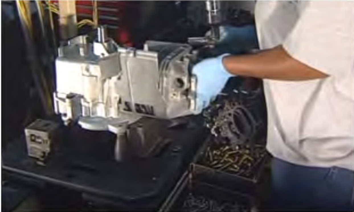
Figure I-7 SVSEs: Head fitted to the cylinder block
