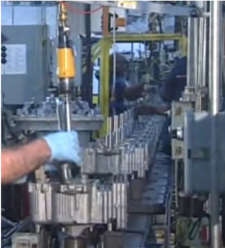
Figure I-5 SVSEs: Crank shaft assembly inserted into the cylinder box
