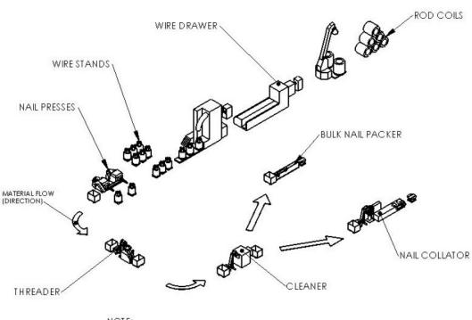
NOTE: ALL COLLATED NAILS ARE VINYL COATED IN-LINE ON THE COLLATING MACHINE. ALL BULK NAILS ARE COATED IN-LINE AT THE CLEANING STATION IF REQUIRED
