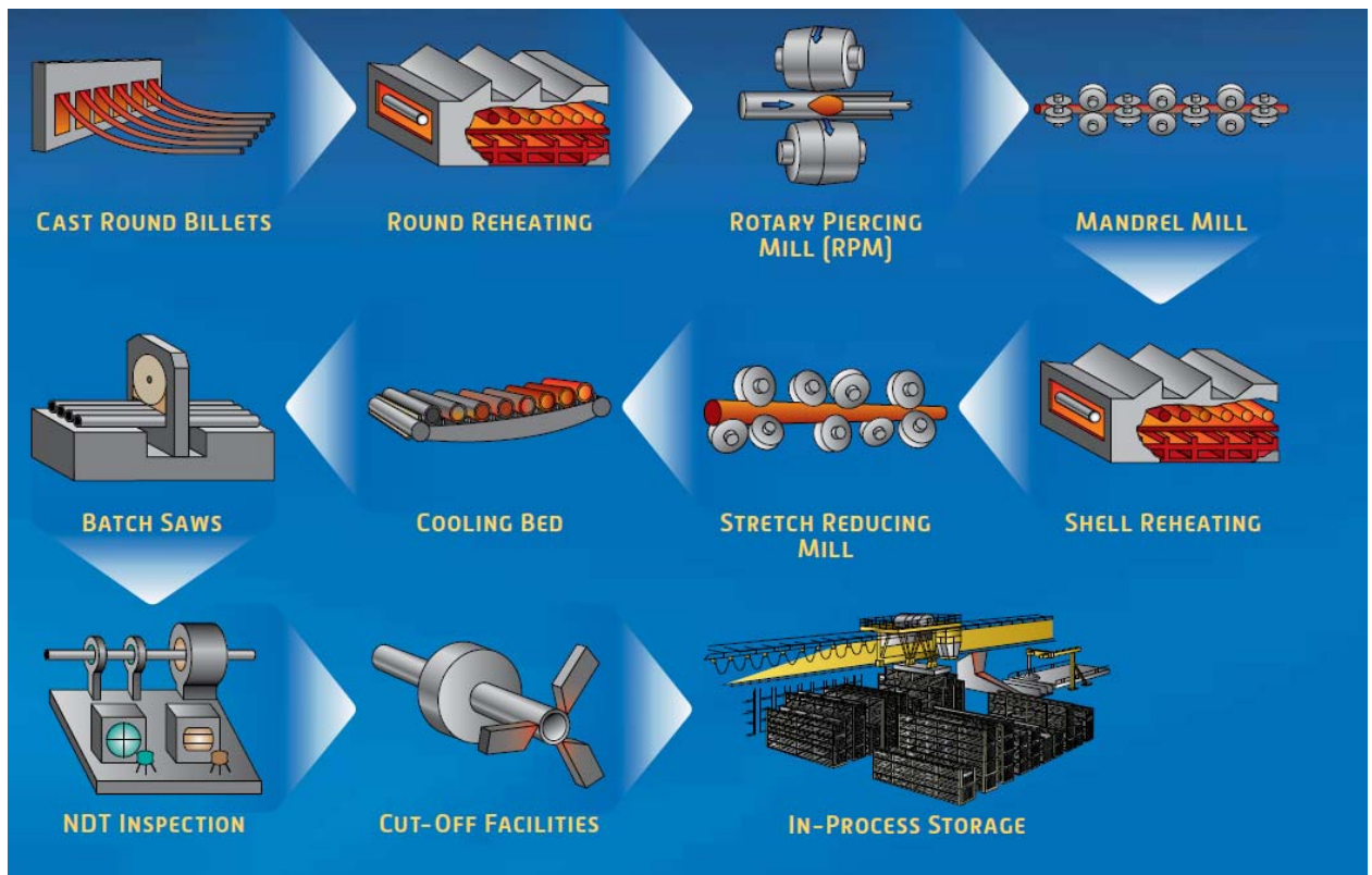
Figure I-1 Seamless pipe: Sequence of operations used to produce seamless pipe products by piercing and rolling
