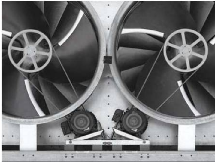
Figure I-9 IMTDCs: Belt drive in an HVAC application
