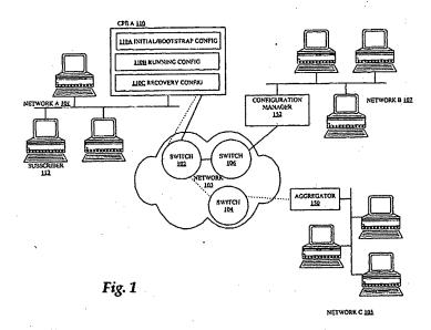
As recited in claim 1, the network device will detect a loss of connectivity between the device and a network (e.g., Networks A [item 101], B [item 107], or C [item 107]) resulting from the configuration change and revert to a recovery configuration ("Recovery Config" [item 110C]).
