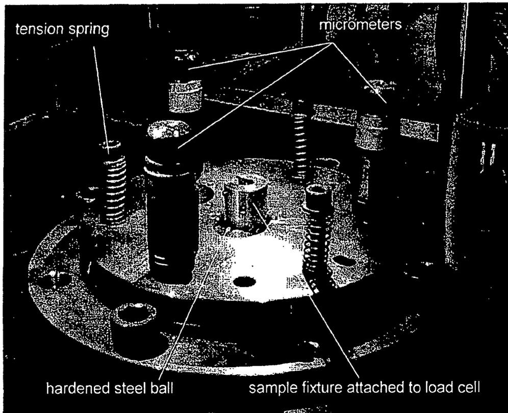
(JX-0004 Photograph 2 (mechanism used to achieve parallelity)).
