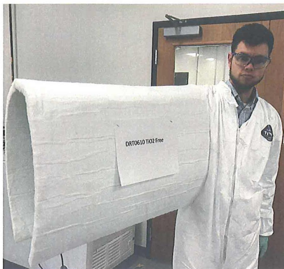
Figure 47: Photograph Showing that Complainant's DI Aerogel Composite Blankets Are Flexible and Light-Weight
