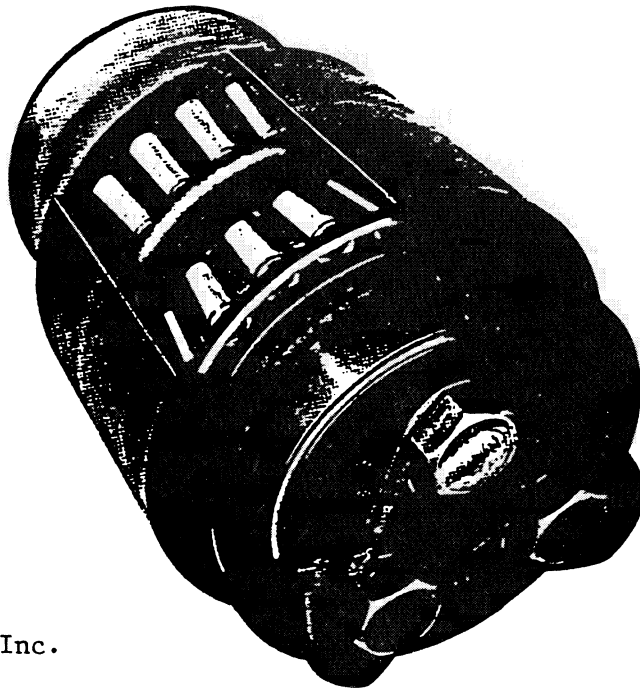
Figure 2.— Principal components of a railway freight car journal roller bearing
