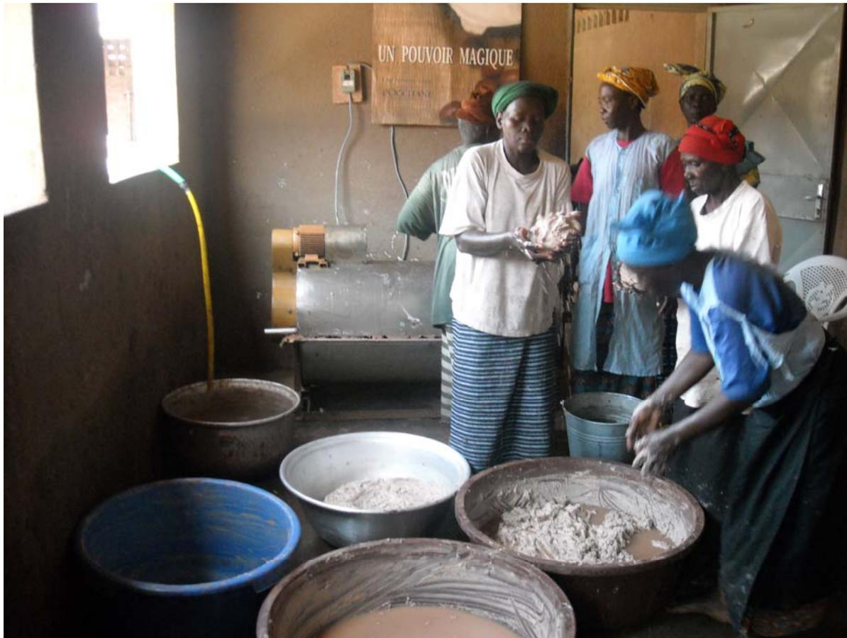
Shea butter producers in Ouagadougou, Burkina Faso, perform hand-kneading operations (foreground), and have one machine to perform electrically powered kneading (background). Burkina Faso's electricity is among the costliest in the world. Relatively less expensive electricity would lead to substitution of mechanized kneading for hand kneading.
